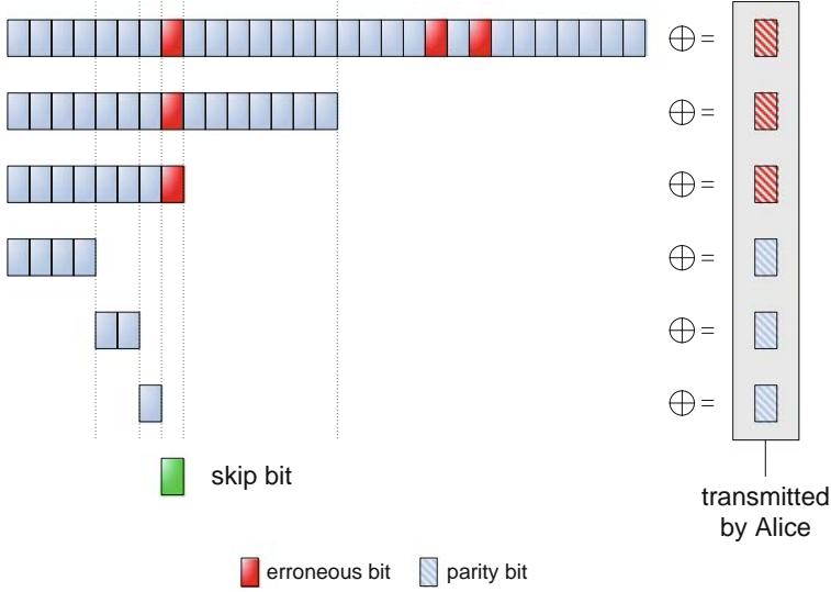
Fig. 3.6 BINARY corrects exact one error of a block with an odd number of errors
